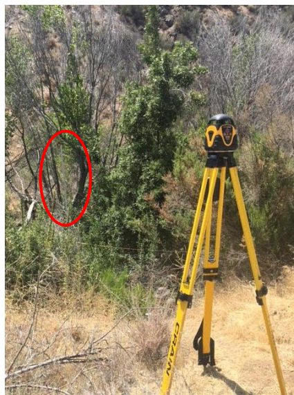
Figure 3. Surveying tool—laser level and measuring rod (red polygon).
